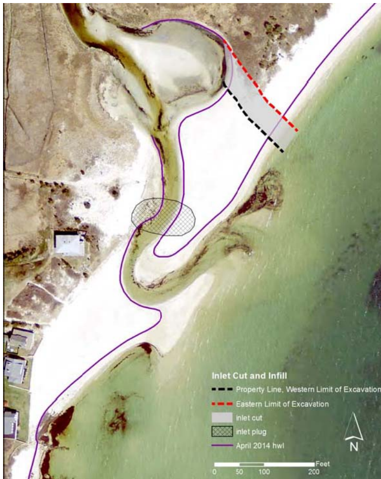
Figure 4: Aerial view of the Meadow Shores Marsh existing inlet and approximate locations of proposed repositioned inlet channel and sand-fill plug in existing channel
